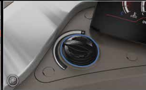
Hand Throttle with Electronic Rotary Control (*)
